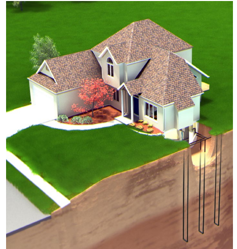
▲ Geothermal heat pumps transfer heat from the ground to your home and can reduce home energy use by 70% to 80%. Photo courtesy of WaterFurnace International.
